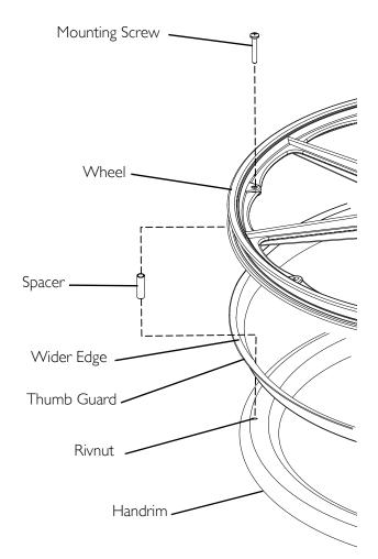
FIGURE I Removing/Installing Handrims with Rivnuts®
